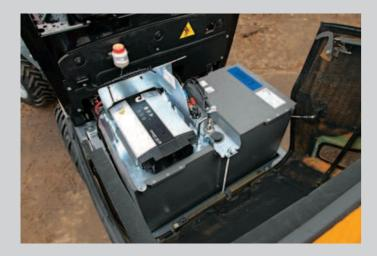
The G2700E models are easy to maintain because service points are easy to access. Hydraulic system and battery are freely accessible via the easy-to-use open service valves. This ensures that daily checks and maintenance can be carried out quickly and safely way can be performed.
